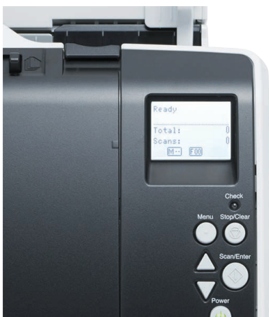
Integrated backlight enhanced LCD operating panel
