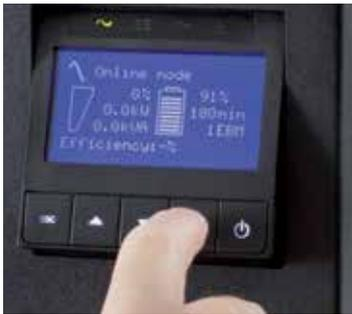
9SX LCD tilts 45° for ease-of-viewing
