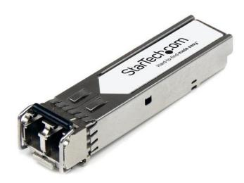
The J9151E-ST is a HP J9151E compatible fiber transceiver module that has been designed, programmed and tested to work with HP brand switches and routers. It delivers dependable 10 GbE connectivity over fiber cable, for 10GBase-LR compliant networks, with a maximum distance of up to 10 km (6.2 mi).
