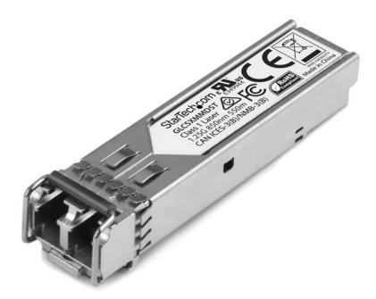
The GLCSXMMDST is a Cisco GLC-SX-MMD compatible fiber transceiver module that has been designed, programmed and tested to work with Cisco® brand switches and routers. It delivers dependable 1 GbE connectivity over fiber cable, for 1000BASE-SX compliant networks, with a maximum distance of up to 550 m (1804 ft).
