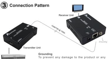
connecting devices, and to improve audio/video signal quality, it is important to make sure that the extender systems are properly grounded.
