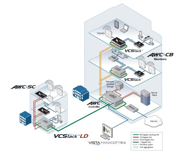
Allied Telesis Autonomous Wave Controller (AWC) offers solutions for two of the most common problems with Wireless LANs: initial setup complexity and on-going performance degradation. Initial WLAN set-up usually requires a site survey to achieve the best coverage; and performance of WLANs can often change over time as external sources of radio interference reduce coverage and bandwidth. These issues can be time-consuming to identify and resolve.
