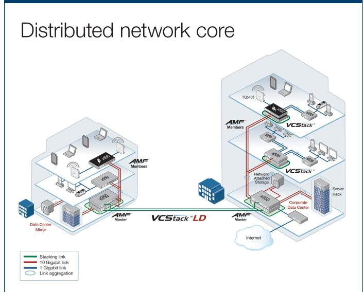
Today's corporate network users demand a high-performing enterprise network that can seamlessly carry multiple converged services, and provide instant access to online resources and applications. This key solution uses the x950 Series and long-distance Virtual Chassis Stacking (VCStack-LD)—ideal for a distributed business network core that provides high availability, increased capacity and ease of management.
