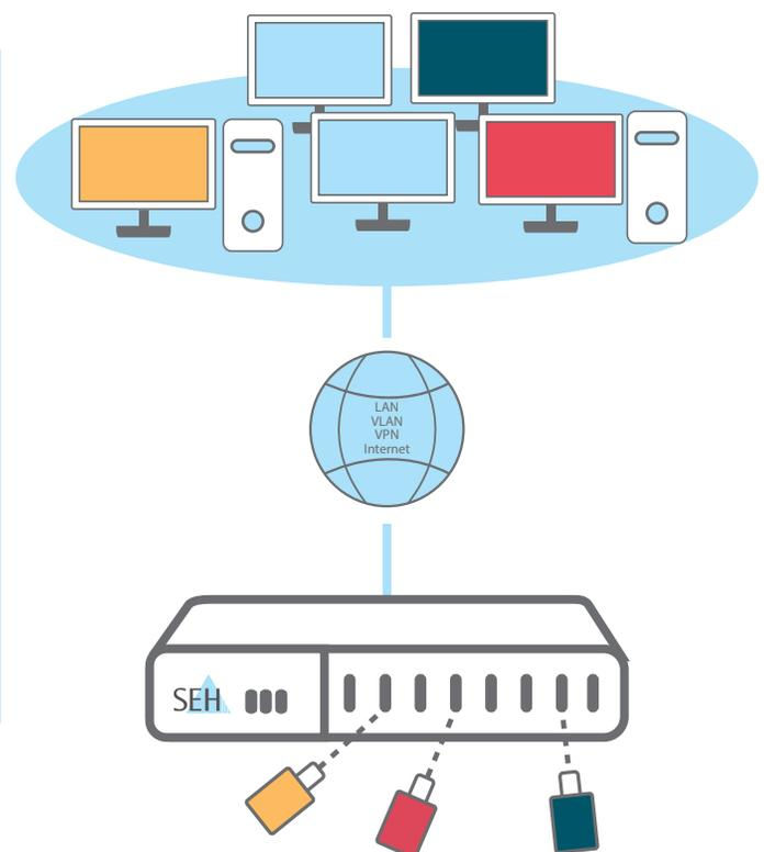
*Dongle servers provide an exclusive point-to-point connection via the network. The working principle of USB dongles as copyright protection is not changed, bypassed or eliminated at any time.*
