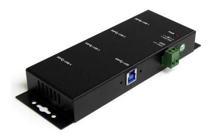
The ST4300USBM Mountable 4-Port Industrial USB Hub (USB 3.0) offers a simple way to expand a systems current USB capability by providing 4 additional external USB 3.0 ports from a single USB 3.0 host connection, with speeds up to 5 Gbps.
