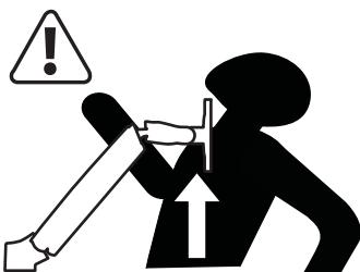
**[EN]** WARNING! Stored Energy Hazard: The arm mechanism is under tension and will move up rapidly, on its own, as soon as attached equipment is removed. For this reason, DO NOT remove equipment unless the arm has been moved to the highest position! Failure to follow this instruction may result in serious personal injury and/or equipment damage!
