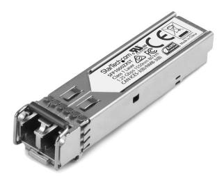
The SFP1000ZXST is an MSA compliant fiber SFP transceiver that's designed, programmed and tested to work with 1000BASE-ZX compatible MSA switches and routers. The SFP transceiver module supports a maximum distance of up to 80 km (49.7 mi) and delivers dependable 1 GbE connectivity over fiber cabling. <br/>
