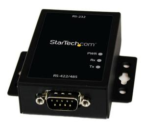
The IC232485S Industrial RS232 to RS-422/485 Serial Converter is a bi-directional adapter that lets you adapt an RS232 data signal to either RS485 (2 or 4-wire) or RS422 and vice-versa, with support for baud rates up to 921.6 Kbps.
