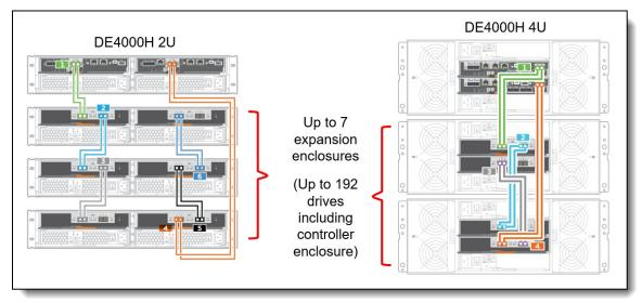
Figure 9. DE Series expansion enclosure connectivity topology
