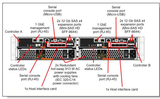
The following figure shows the rear of the ThinkSystem DE4000H 2U controller enclosure.
