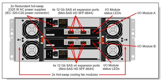
The following figure shows the rear of the ThinkSystem DE600S 4U LFF expansion enclosure.
