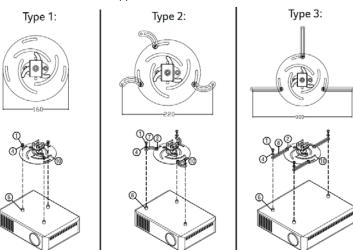
Connect the main body connector to the projector bracket (illustration 1), and then screw up four screws (illustration 2).
