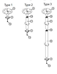
Type 1: For the standard size use three bracket screws to mount the projector to the ceiling mount bracket.
