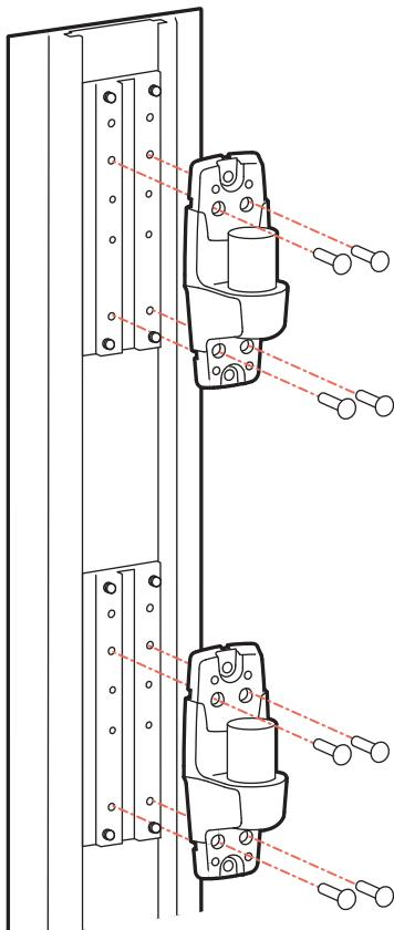
**EN** NOTE: Fasteners may unwind due to vibration caused by movement of mounting solution over time. Inspect mounting solution for loose fasteners on a routine basis. If desired, apply a light duty thread locking adhesive to fasteners before installation to prevent back-out.
