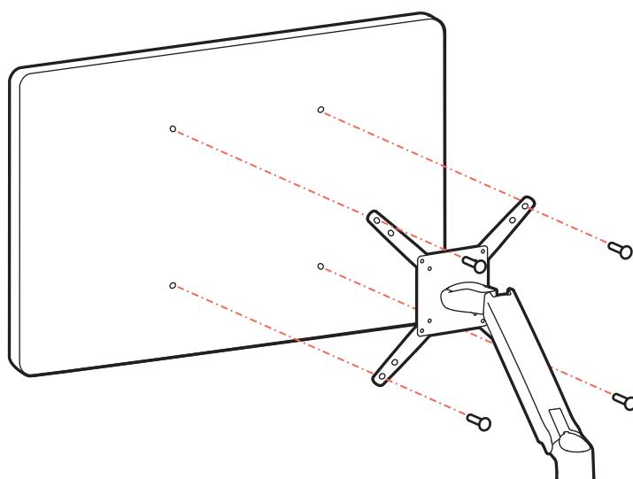
NOTE: To reduce M8 holes for use with M5 screws, or if you have a model with Samsung holder rings, follow the M8M5 KIT instructions on the next page.
