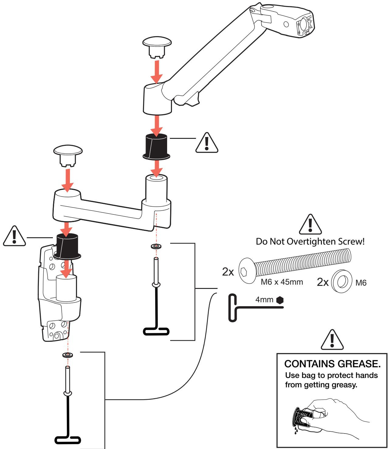
NOTE: when sliding sleeve on to bracket, align slot over rotation stop.
