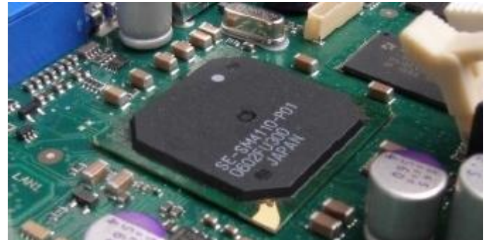
iRMC S4 – integrated Remote Management Controller
