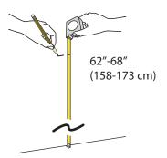
Level and secure template to the wall lining up the chosen mounting holes with the mark 62"-68" (158-173 cm) from floor.
