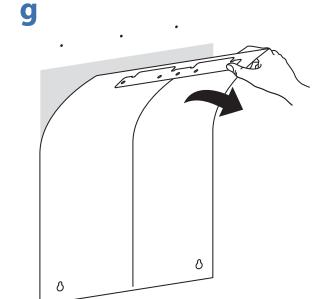
Insert anchors then attach bracket to wall according to the hole option determined on previous page. Verify wall bracket is level before tightening screws.
