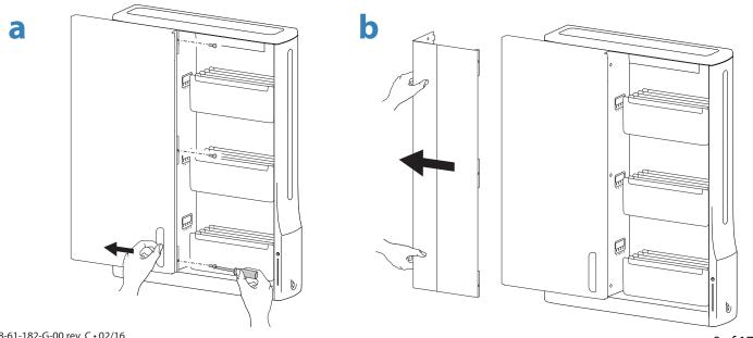
a. Secure unit to wall by inserting screw through back wall and into bottom right wall anchor.
