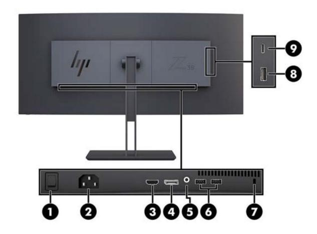
1. Master power switch Turns off all power to the monitor
