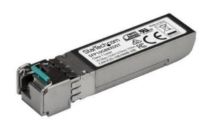
The SFP10GBBXDST is an MSA compliant downstream fiber SFP transceiver which pairs with StarTech.com's SFP10GBBXUST. They are designed, programmed and tested to work with 10GBASE-BX compatible MSA switches and routers. The SFP+ transceiver module supports a maximum distance of up to 10 km (6.2 mi) and delivers dependable 10 GbE connectivity over fiber cabling.
