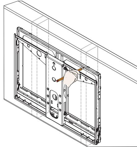
Use a pencil to mark the upper right mounting location of the wall stud.
