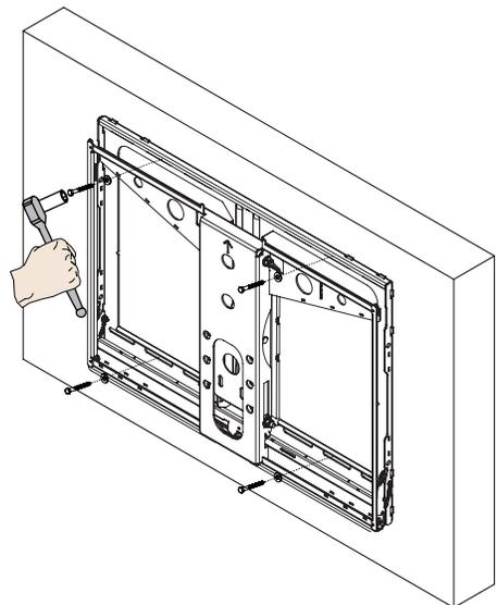
1. Insert one (1) 5/16" x 3" Lag Bolt and one (1) 5/16" washer into each pilot holes.
