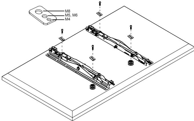
Universal Washers are designed to accommodate the various M4, M5, M6 and M8 hole sizes required by flat-panels.
