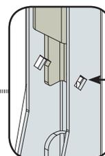
**Note:** These registers must align prior to installation. They are factory set. Check to determine proper alignment
