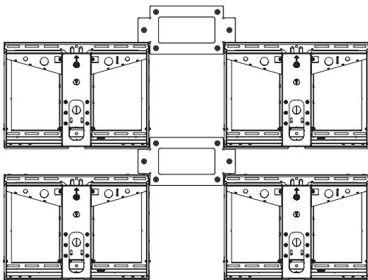
Multiple PFW6880 mounts can be installed using model specific spacers. Simply repeat step one when installing each of the surrounding PFW6880 mounts. Use one spacer for each 2x2 installation by mounting it to the wall, or utilize the same spacer as many times needed to complete an unlimited PFW6880 large matrix video wall.
