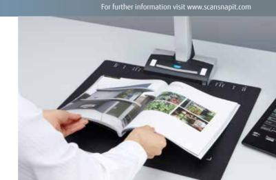
Bound documents can be scanned by the SV600 with the enhanced ability to continuously scan multiple pages without delay. The SV600 features page turning detection and timed mode to scan again after a set time. Further book scanning features include book image correction which automatically corrects any distortion caused by the curve of an open book and a user interaction retouch function.
