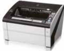
The fi-6800 also offers superb capture reliability and image processing. Impressive scanning speeds help set the fi-6800 apart. At 300 dpi in A4 landscape mode 130 pages per minute can be achieved whether scanning in mono or colour. This is doubled to 260 images per minute in duplex. The ADF hopper can take a maximum 500 sheets.
