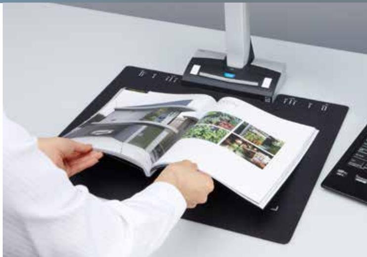
Bound documents can be scanned by the SV600 with the enhanced ability to continuously scan multiple pages without delay. The SV600 features page turning detection and timed mode to scan again after a set time. Further book scanning features include book image correction which automatically corrects any distortion caused by the curve of an open book and a user interaction retouch function.
