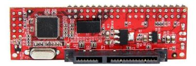
The IDE2SAT2 40-pin IDE to SATA adapter enables you to connect a SATA I/II/III drive to an available IDE/ATA 33/66/100/133 motherboard port - a cost effective solution that allows you to add newer SATA drives, and keep your existing motherboard.
