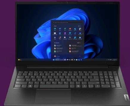
The HD 2W dual Realtek® ALC3287 codec speakers provide a rich, immersive sound experience, enabling professionals to collaborate seamlessly with colleagues and clients, even while on the move. Furthermore, the dual-microphone array guarantees clear voice transmission during video calls and conferences.
