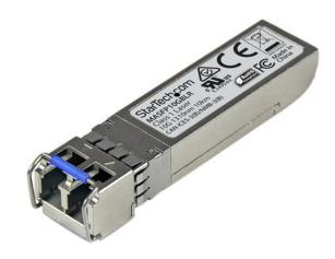
The MASFP10GBLR is a Cisco Meraki MA-SFP-10GB-LR compatible fiber transceiver module that has been designed, programmed and tested to work with Cisco Meraki<sup>™</sup> brand switches and routers. It delivers dependable 10GbE connectivity over fiber cable, for 10GBASE-LR compliant networks, with a maximum distance of up to 10 km (6.2 mi).
