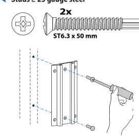
NOTE: Fasteners may unwind due to vibration caused by movement of mounting solution over time. Inspect mounting solution for loose fasteners on a routine basis. If desired, apply a light duty thread locking adhesive to fasteners before installation to prevent back-out.
