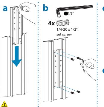
NOTE: Fasteners may unwind due to vibration caused by movement of mounting solution over time. Inspect mounting solution for loose fasteners on a routine basis. If desired, apply a light duty thread locking adhesive to fasteners before installation to prevent back-out.
