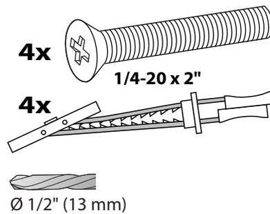
**⚠** Requires minimum material thickness of 5/8" (16 mm).
