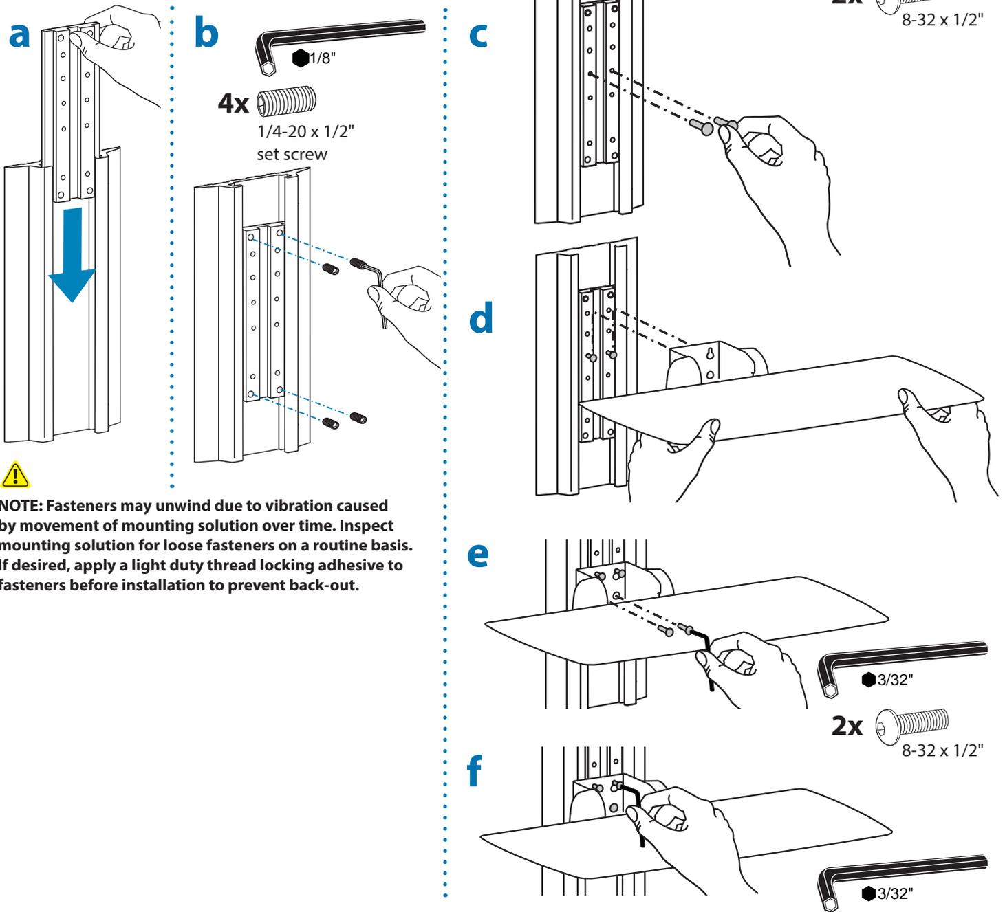
**NOTE:** Fasteners may unwind due to vibration caused by movement of mounting solution over time. Inspect mounting solution for loose fasteners on a routine basis. If desired, apply a light duty thread locking adhesive to fasteners before installation to prevent back-out.
