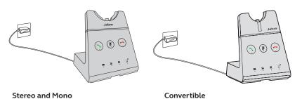
Plug the base into a power supply. Press Vol + and Vol - simultaneously to enter the setup menu to help you connect to your computer or desk phone.
