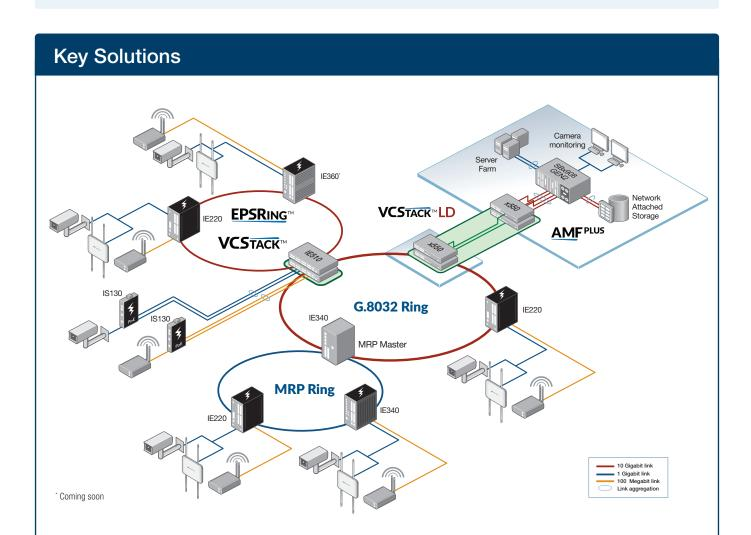
Media Redundancy Protocol (MRP), EPSRing and ERPS (ITU G.8032) provide high-speed resilient ring connectivity. This diagram shows how the IE Series can support a variety of ring network topologies.
