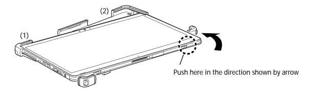
4. Fit the lower side of the tablet into the Bumper Case.
