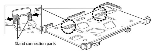
3. Use alignment mark as a reference and fix the stand spacer to the empty space.
