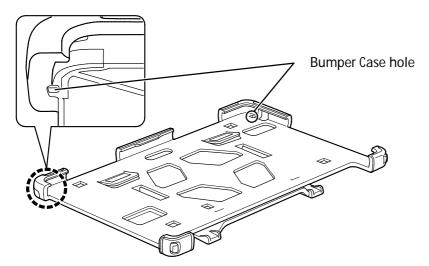
3. Fit the upper left side of the tablet into the upper left side (1) of the Bumper Case, move the tablet in the direction of the arrow and fit it into the upper right side (2) of the Bumper Case.
