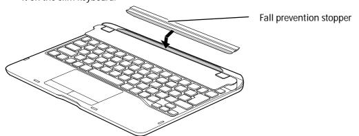
Paste it firmly. After pasting, please do not apply force to the fall prevention stopper for about one day to ensure the adhesive strength.
