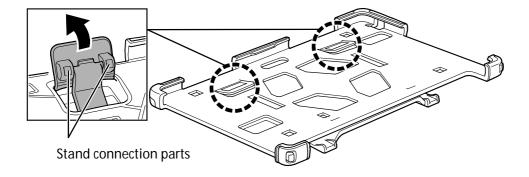
2. Expand the stand connection parts in the direction of arrows shown in the following figure and then remove the stand.
