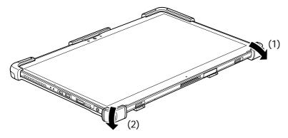
Remove the tablet from the Bumper Case.
