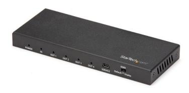
This 4-Port 4K HDMI splitter connects your HDMI video source to four HDMI displays at the same time, without distorting or degrading your video signal. For dependable performance, the splitter features a durable metal housing that provides passive cooling.
